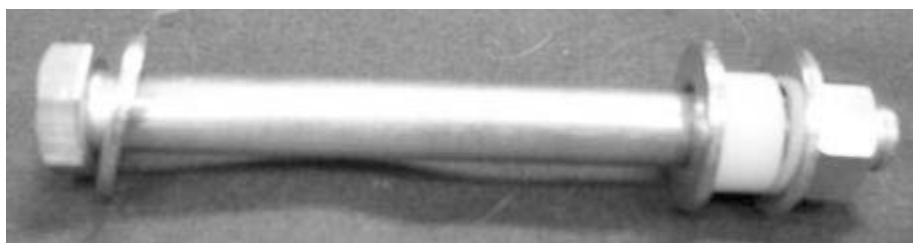
FIGURE 28 - Axle Assembly for Attaching the Wheels to Frame.
