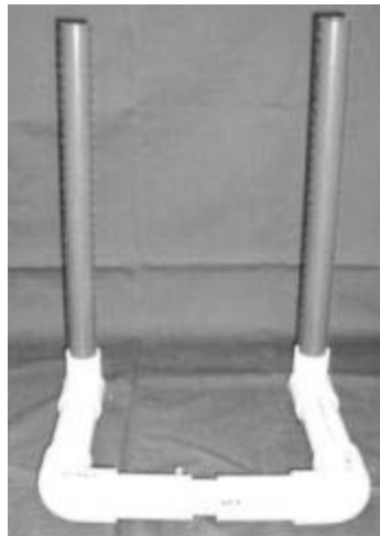
FIGURE 23 – Step 18 – Joining Side Frame to Rear Frame.
