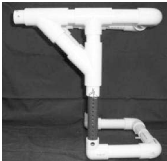
FIGURE 26 – Side View of Wheelchair Frame Subassembly.
